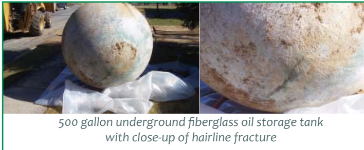
Underground Oil tank removal after evidence of leaking
