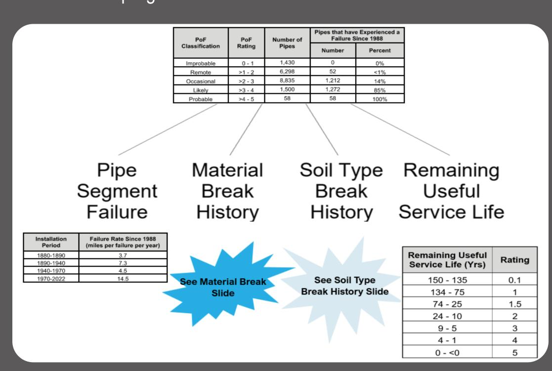
Characteristics such as pipe segment failure, material break history, soil type break history, and remaining useful service life were observed and used to create Asset Risk Exposure Assessment (AREA) ratings for sections of the system.
